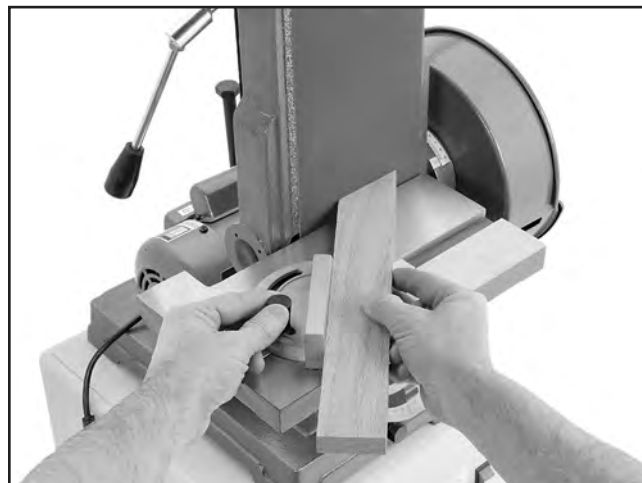
Figure 73. Example of vertical miter sanding.
